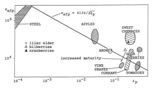
Fig. 2. Critical values of effective stress ( $\sigma_{efp}$ ) in relation to critical values of relative compression ( $\varepsilon_p$ ) for different agricultural round products and steel spheres. Critical point is identified with the beginning of anelastic behaviour of the compressed product and/or sphere in this case.
