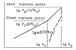
Fig. 3. Schematical drawing of a typical compression curve of a berry-like fruit compressed between two plates (full line). Function log  $[(F-\Delta F)/(2\pi r_0)]$  is denoted by the dashed line.
